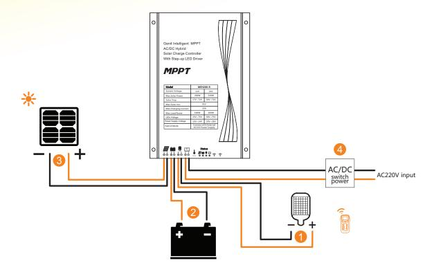
A Wiring sequence: Please connect the load first, then the battery, then the solar panel, and finally the DC. Please don't connect 220V AC directly to the controller!
